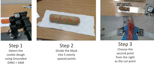
Fig. 5. Breakdown of the Perception stack of the Cutting task. First, the segmentation mask of the cookie dough is obtained from the wrist-camera (left). Next, a sequence of N evenly spaced cut points are obtained (middle). Finally, the second point from the right is selected and passed to Cutter for control (right).
